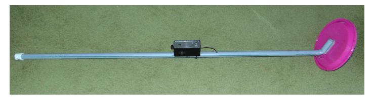
The complete metal detector "stick" is shown above. It's easy to wave this around and scan for metallic objects.
