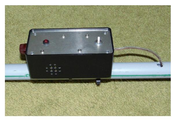
Here is an expanded image of the control box enclosing the PIC circuit on the 2 layer PCB, the piezo speaker. As well I added an earphone jack, and a series variable resistor to control earphone audio.
