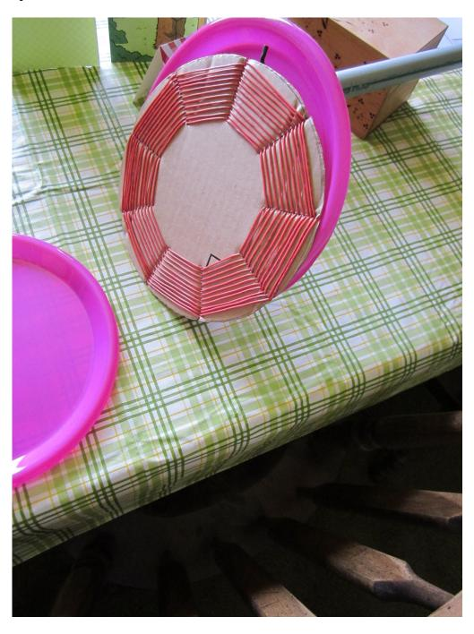
Note that the coil is mounted between 2 plastic dinner plates on the end of a PVC pipe. The coil is woven on an 9 inch diameter cardboard disk with 9 (equidistant) slots cut into it. By doing an odd number of slots, weaving in and out around the circumference causes odd and even turns to have the opposite weave, thus minimizing capacitance between windings. The coil has 23 turns on it, of AWG no. 20 stranded wire with plastic insulation.
